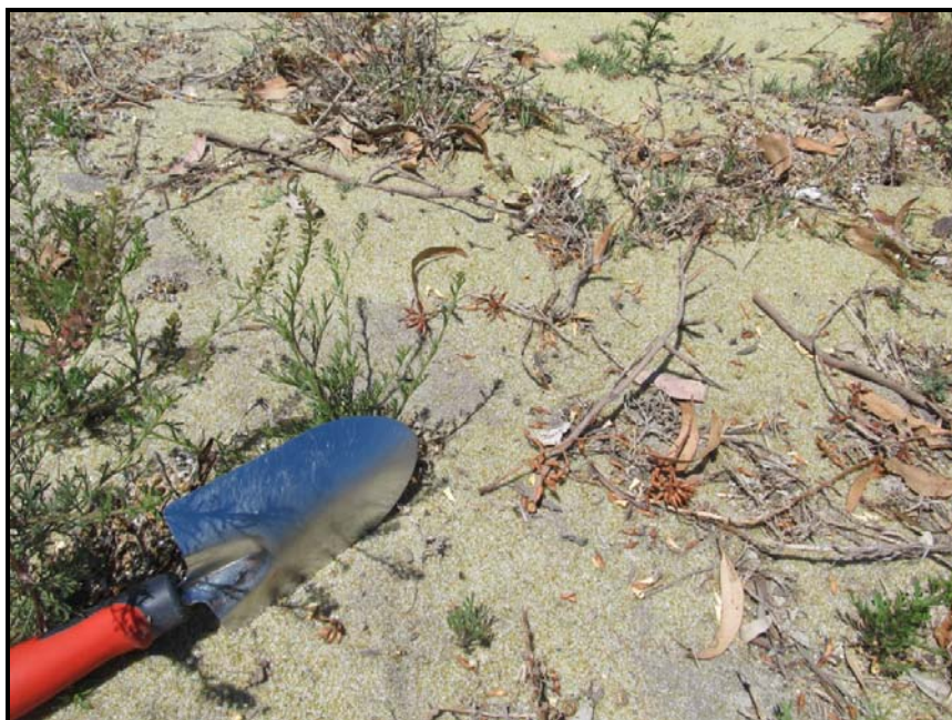
Photo 8: Photograph of ground surface on horse track on Lot 536 showing ACM fragments.
